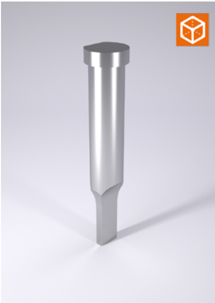
2251. Punch, stepped, rectangle with radiused corners, ISO 8020
